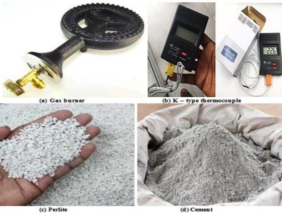
Figure 1: Furnace accessories and refractory materials
